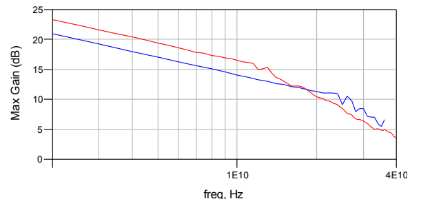
Fig 3. MSG/MAG gain of AlInN/GaN device (red) and, AlGaN/GaN device (blue).
