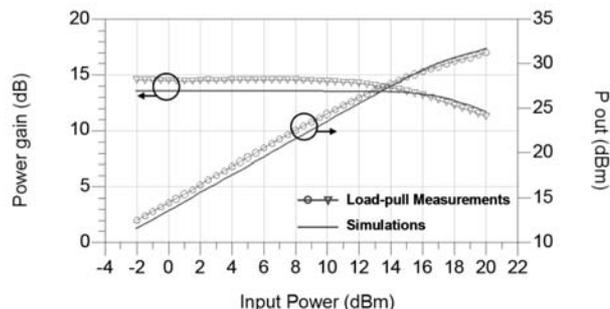
**Fig. 10.** Comparison between simulated and measured large signal results for the cascode cell @ 10GHz.
