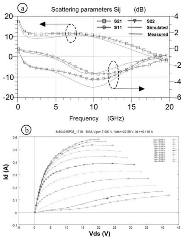
**Fig. 8.** (a) : Simulated and measured S-parameters of the cascode cell. (b) : Pulsed I-V Characteristic of 8x50µm device measured at the quiescent bias point ( $V_{gs0}=-7V$ ,  $V_{ds0}=22.6V$ ).
