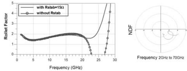
**Fig. 4.** Influence of  $R_{stab}$  on Rollet factor and NDF of the cascode cell.
